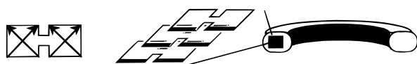
Figure 2. Schematic representation of the porphyrin wheels constructed from porphyrin 1 . The arrows indicate the transition dipole moments of the porphyrin molecules in the dimers. The two sets of dipole moments in a dimer make an angle of \alpha = \pi/4 with neighboring sets of dipole moments, which results in a red shift of the porphyrin B-band. 9
